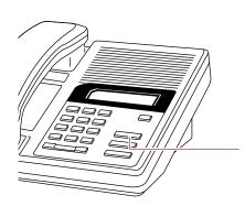
The memory key can store a telephone number or feature code to give you one touch dialling or feature activation. You can change the memory key by programming it with a new number or feature code.
